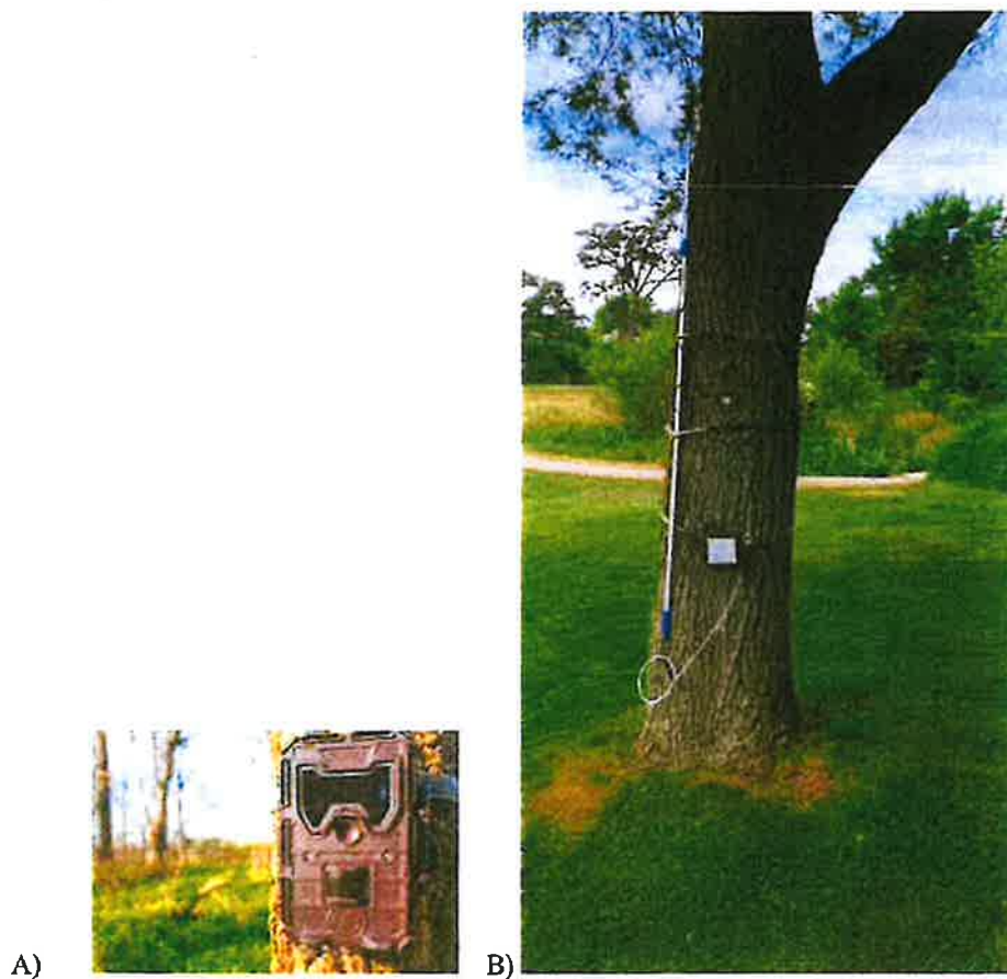
Figure 1. A) A trail camera attached to a tree. B) An ultrasonic recorder secured with a bungee cord and equipped with an ultrasonic microphone extended on a pole.
